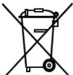
The instrument contains a lithium battery for memory back-up (saving the data). When exceeding the specified minimum battery voltage or in case of defect, the battery must be replaced by the SARTORIUS customer service or by an equivalent trained person and disposed of in accordance with the local regulations.
