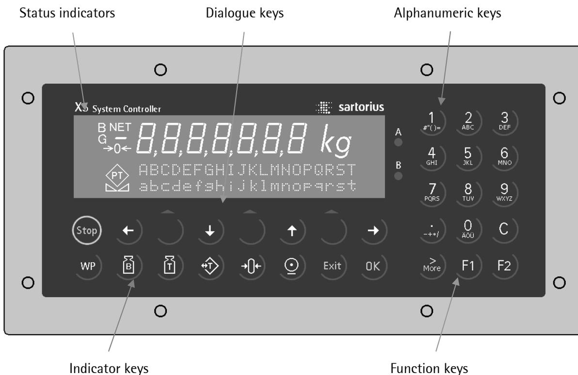
The **Weight Display** allows display of 7 digits for weight plus a decimal point. The unit can be selected as tons, kilograms, grams or lbs. The display is capable of handling two lines of text in addition to the numeric output. The other symbols in the display are listed below:
