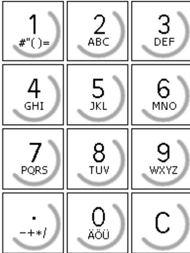
The alphanumeric keys have got more than one assignment. After pressing for the first time, the relevant first character, e.g. 'A' is displayed in the cursor position. After pressing for the second time, e.g. 'B' instead of 'A' is displayed; 'C' is displayed after pressing for the third time, etc. After the last signification, the first one is displayed again. Pressing another character key, or the right arrow key completes the entry of a character.
